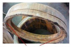
Fatigue crack on on outer ring raceway surface center
